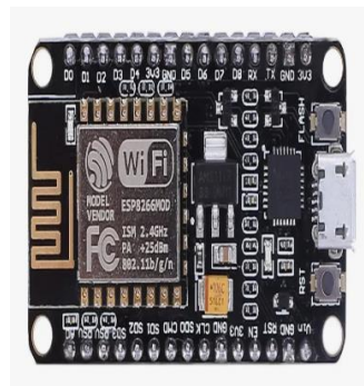
Figure 8- Full-fledged platform based on the ESP8266 module
